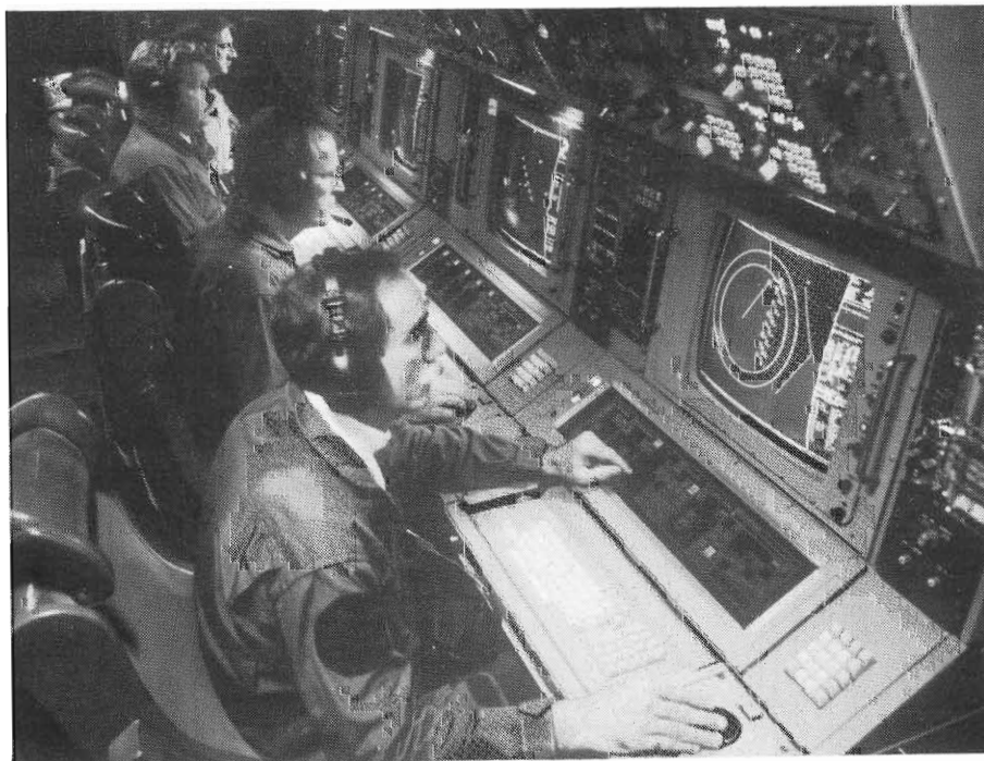
The Universal Display and Control System (UDACS) workstations are a key element in the US Navy's P-3 Update IV system. The first functional flight test of the Update IV system, developed by Boeing Defense and Space Group, took place on 16 December 1991.
