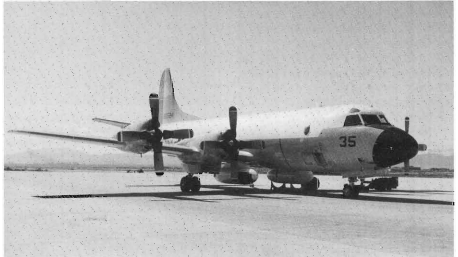
Naval Air Warfare Center Weapons Division (NAWCWPNS), Test and Evaluation Support Aircraft Division (P355) RP3A aircraft Buno 150524, Bloodhound 35 (BH35) with POD 1, the Synthetic Aperture Radar (SAR) POD loaded on Station 15, and POD 2, the Multispectral Imaging (MSI) POD, loaded on Station 12. (INFOTEC)
