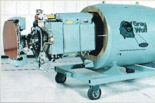
AN/APN-76 Radar installed in a modified S-3 cargo pod for the Gray Wolf Proof-Of-Concept Project. The original nose of the pod was replaced with an F-4 nose cone.
