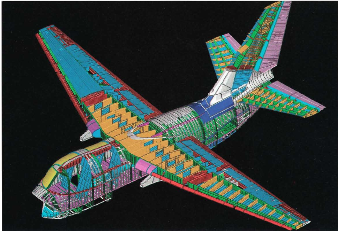
On the S-3 airframe Finite Element Model or FEM, 22,784 grid point locations were generated from aircraft loft lines and used to form a computer generated mesh of 50,294 finite elements which represent all load-bearing structure. The goal is to calculate stress levels and help locate fatigue problem areas.
