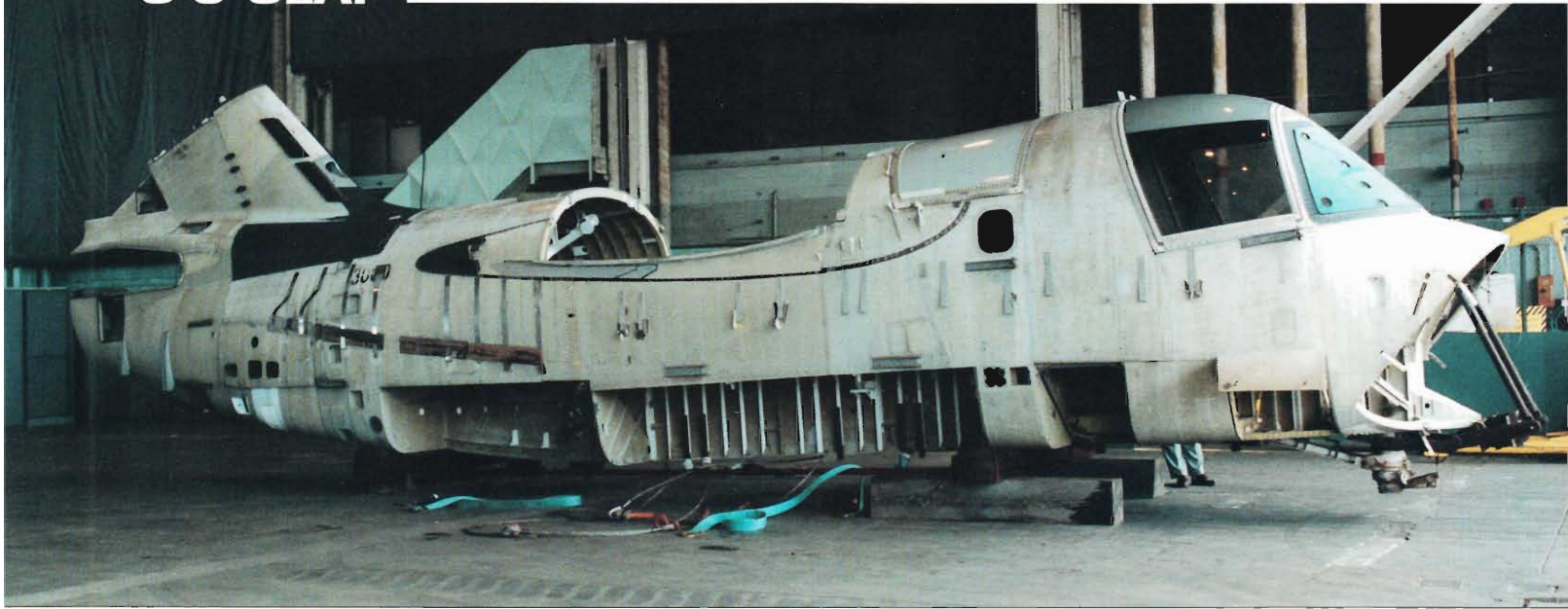
The original S-3 fatigue test article, known as Ship 3000, as it appears today in a Lockheed hangar. It was almost scrapped after its first fatigue testing program, and has proved essential to the SLAP tests.
