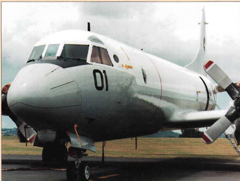
Radome experimentation by the RNZAF is an attempt to reduce moisture ingress.
