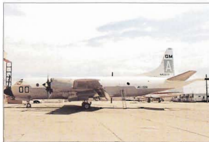
151391 as Allison GMA 2100 Engine Testbed Orion
