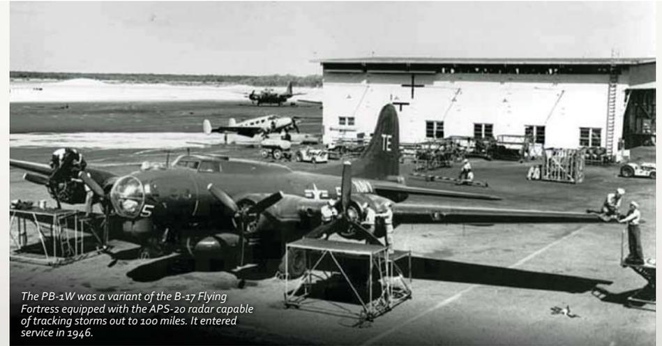
The PB-1W was a variant of the B-17 Flying Fortress equipped with the APS-20 radar capable of tracking storms out to 100 miles. It entered service in 1946.
