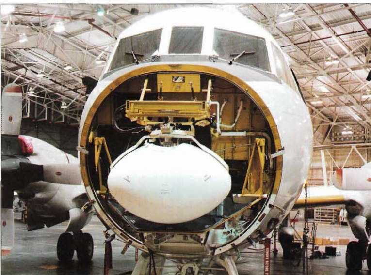
The APS-137 ISAR will replace the APS-115 radar.
