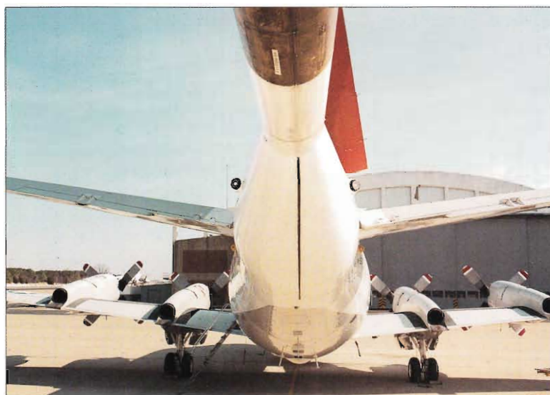
Fore and aft installation of the ARR-47 Missile Warning System
