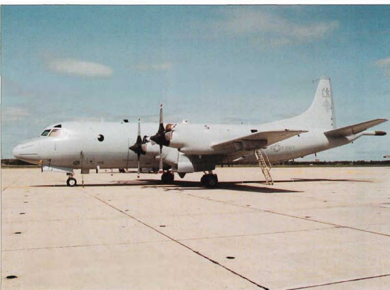
An OASIS II equipped Orion showing the GPS (black) and SATCOM (white) antennas.
