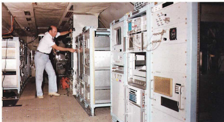
All versatile test bed Orions are equipped with a universal rail system to accommodate avionics systems for testing.
