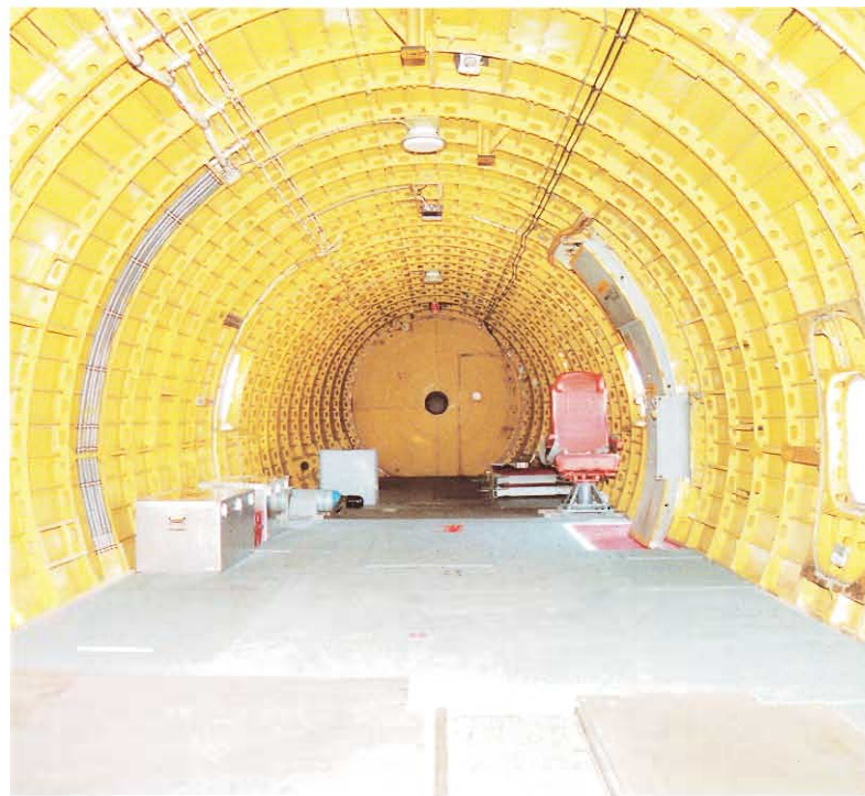
Looking fore and aft in a stripped P-3 can be a real shock. All “non-essential” materials are removed. Aero Union obviously has a very short list of essential equipment. The modification, from arrival to finished and flying, takes only four to six months.
