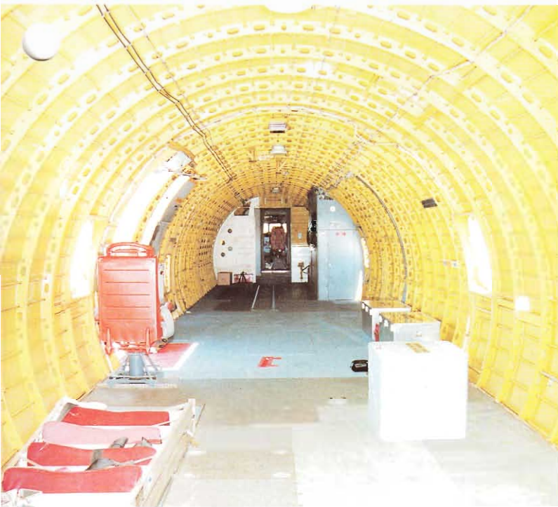
Looking fore and aft in a stripped P-3 can be a real shock. All “non-essential” materials are removed. Aero Union obviously has a very short list of essential equipment. The modification, from arrival to finished and flying, takes only four to six months.
