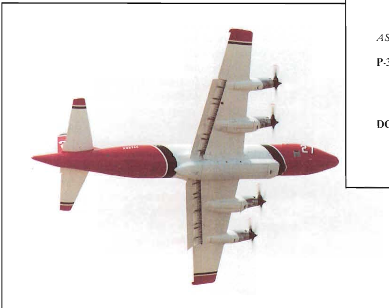
Aero Union sources report receiving a request from a Seattle Company for a bid to convert another batch of bone yard P-3s to oil well fire fighters. Their ultimate destination would be Saudi Arabia. Tanks are fabricated by Aero Union (rt.)
